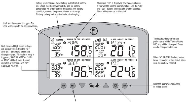
Press to select a probe channel to adjust settings. If no settings are changed after 10 seconds, the display will return to normal.
