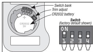
**Switch 1** - *Display Units* - Changes display units between °F (factory default) and °C. To change to °C push the switch toward the batteries.
