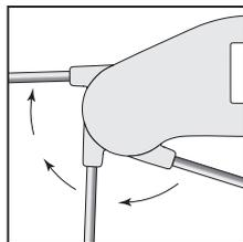
Apply the tip of the probe to the substance, surface or area to be measured. The probe should be allowed adequate time to stabilize to the temperature of the item to be measured.
