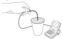
Turn ChefAlarm on and immerse the probe into the ice bath and gently stir. When the temperature is stable and no longer changing, note the final reading. It should be close to 32°F. However, it may be low or high by several tenths of a degree or even one or two whole degrees. If, for example, the reading is 31.4°F, then you are reading low by 0.6°F.
