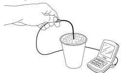
Repeat the ice bath test in Step 1. You should be dead-on or within  $\pm 0.1$ °F.
