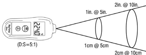
**MEASUREMENT ZONE/TARGET DISTANCE** - The measurement zone is proportional to the distance the RayTemp Blue is away from the target. The RayTemp Blue is equipped with a 5:1 lens. If the target is 5 inches away, the measurement zone will be 1 inch across.
