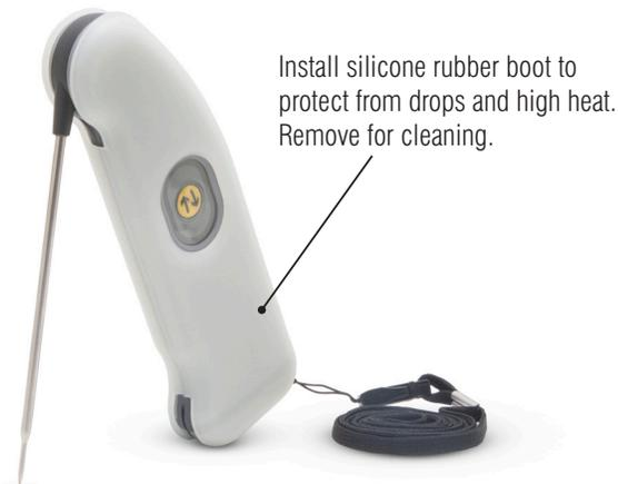
Install silicone rubber boot to protect from drops and high heat. Remove for cleaning.
